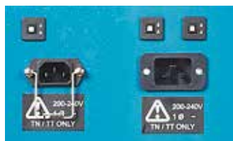
240 Vac domestic electrical connection
